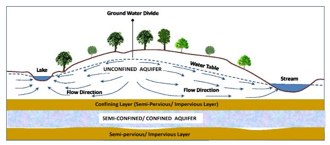
Figure 1.2: Schematic of hydraulic connectivity between water resource types in NRGB
